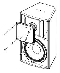
Reassemble the assembly and replace the grille.
