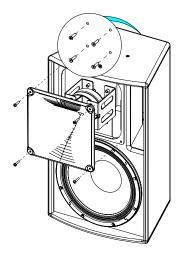
Reassemble the assembly and replace the grille.
