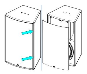
Remove the 4 screws at the back of ePS12-EN54 and the 4 screws that hold the horn. Remove it.
