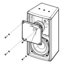
Reassemble the assembly and replace the grille.
