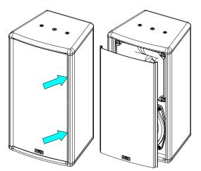
Position the horn according to the desired HF dispersion.
