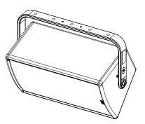
Remove the M10 inserts from each side. Place HBRK425 on ePS8-EN54, use only fasteners provided. Tight properly.
